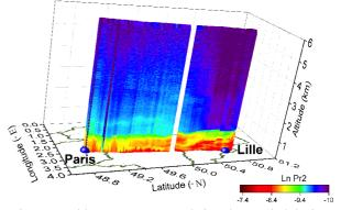
Figure 1. Lidar range corrected signal recorded during Lille-Paris mobile measurements
